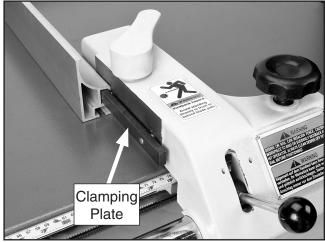
Figure 25. Installing the rip fence.
